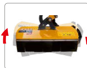
Sistema Floating. Floating head system.
