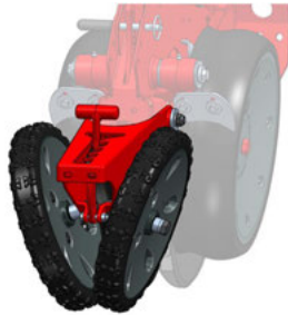
V-pressure wheels wide with profile: for light soils and fine seeds (beet and rape)
