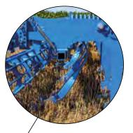
**Levelling harrow** to ensure optimal levelling
