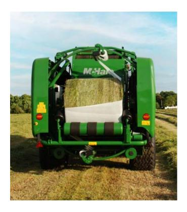
(3) As the bale is forming inside the chamber, the hydraulics take over the tensioning of the belt(s) from the four large springs. Two hydraulic rams control the tension on the chamber belt(s) as the bale forms inside the chamber.
