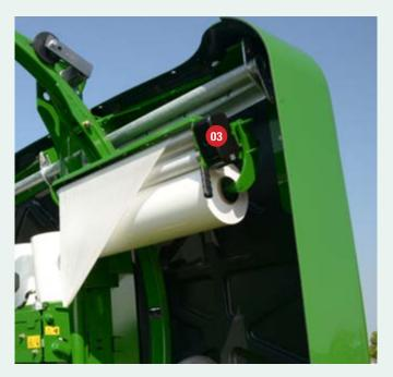
The dispensers are fitted with film break sensors, which notify the operator through the control console in the tractor cab if one or both dispensers run out of film. If one dispenser runs out of film the Fusion Vario will continue working and automatically slow bale rotation and increase the number of rotations of the wrapping ring to ensure that the bale is wrapped correctly.
