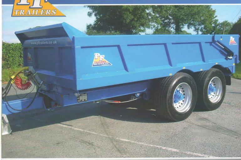
The PF multi-purpose trailer is designed with the user in mind. The trailer is capable of transporting excavators and other machinery. Aluminium ramps are supplied and stored under the trailer bed.
