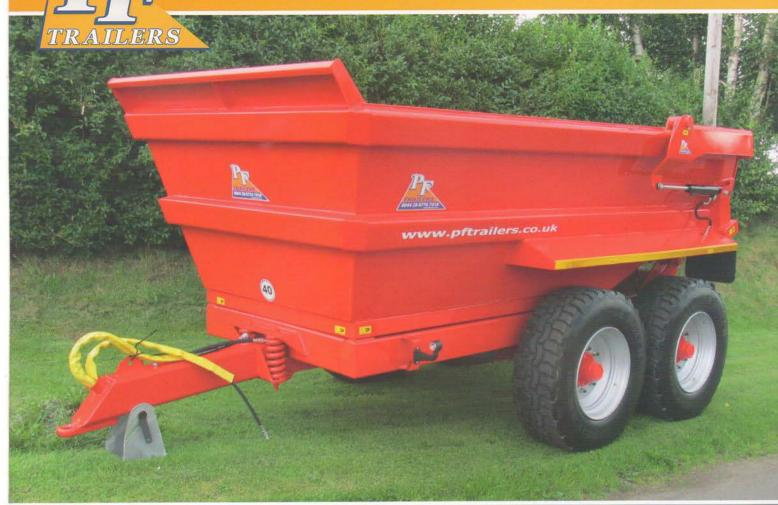
This hydraulic tipping dump trailer comes in either a 12 Tonne, 14 Tonne, or 16 Tonne size.
