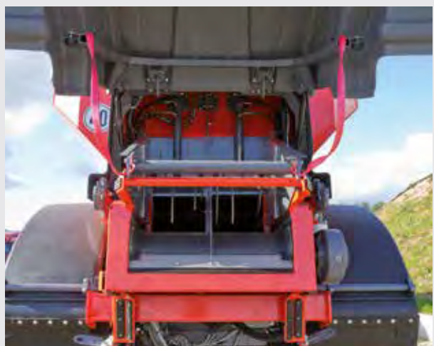
Maintenance flap with gas pressure spring
