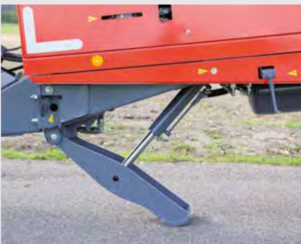
The hydraulic support stand provides quick and reliable stabilisation
