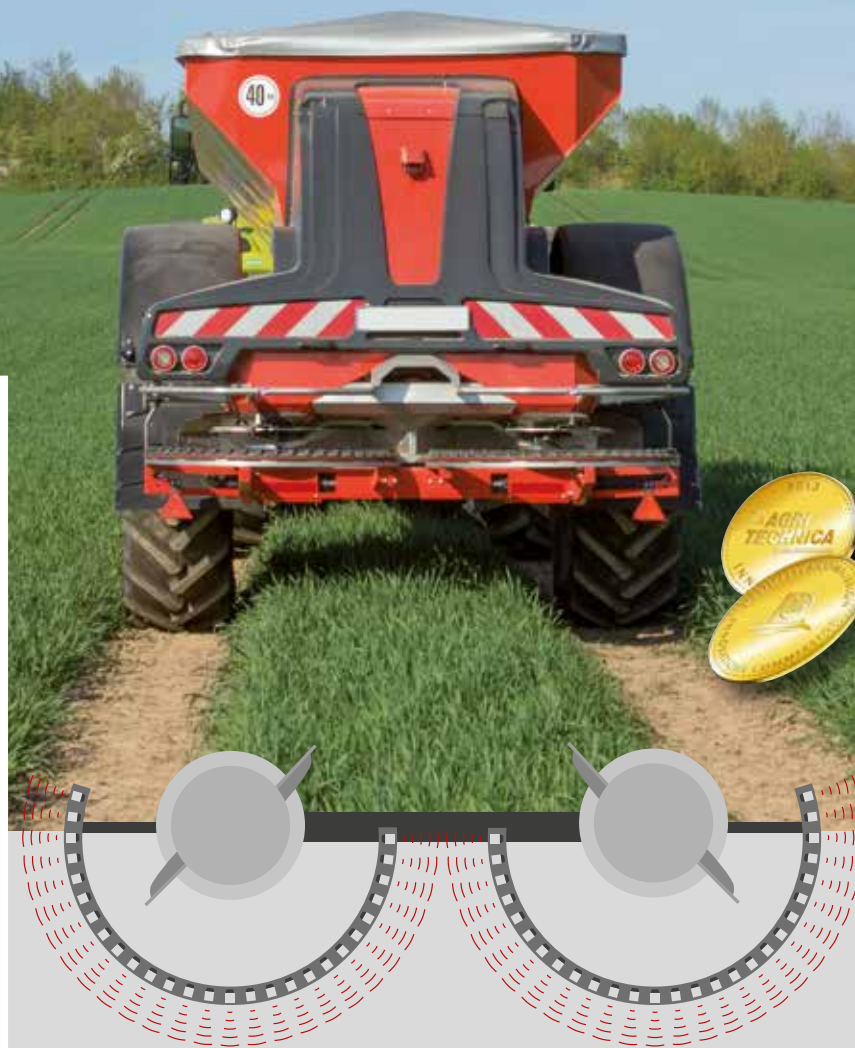
Precise spreading pattern analysis via 54 radar sensors
