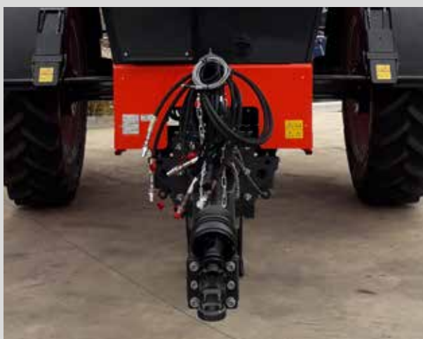
AXENT is optionally available with top or bottom hitching
