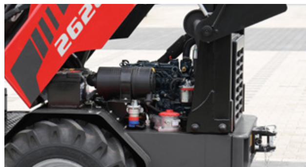
The motor room opens forwards. This makes all service points easily accessible from both sides of the machine.
