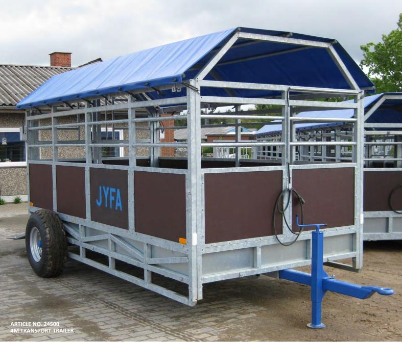
▼ The trailer is equipped with galvanised plates on the inside in the trailer for fast and easy cleaning
