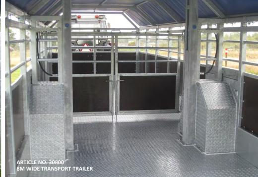
$\checkmark$  If the trailer is equipped with hydraulics, the loading height is 11 cm
