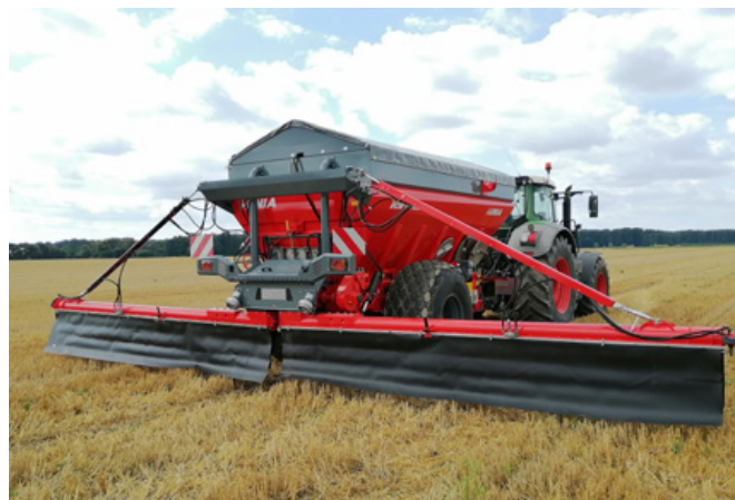
Hydraulic slider (left/right) for even more precise spreading
