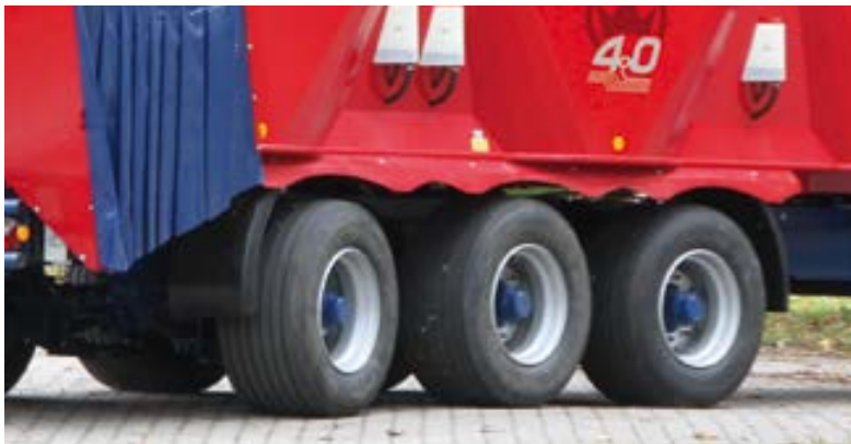
TrailedLine 4.0 System 1000+ 4535-40 / 45 with tridem axle with 2 steering axles as standard.
