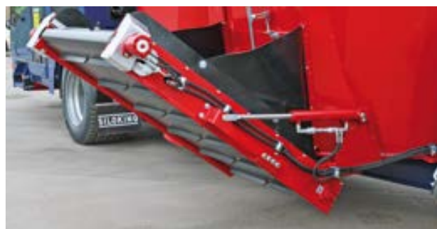
The foldable discharge conveyor belt is used for feed discharge into higher troughs, too.
