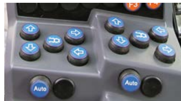
The discharge conveyors are controlled from the driver's cab by simply pushing a button.
