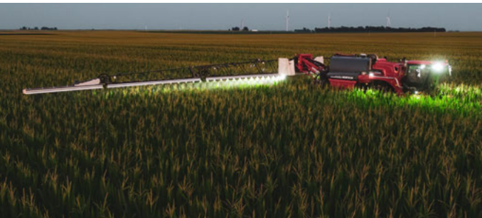
NightLight nozzle cone illumination
