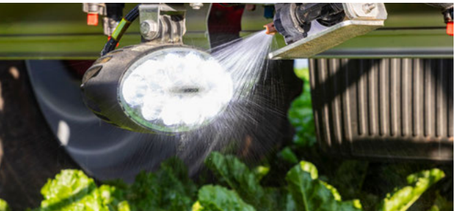
NightLight incl. cleaning
