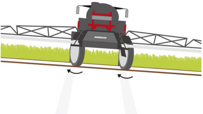
The active hillside counter-steering system HillControl compensates drift on side slopes and ensures a directionally stable following of the rear axle.
