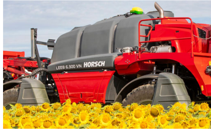
Maximum crop protection with wheel housings for sensitive crops
