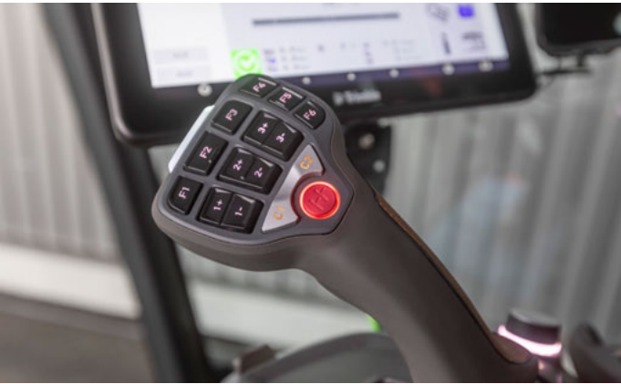
Ergonomic control lever with multiply assignable buttons
