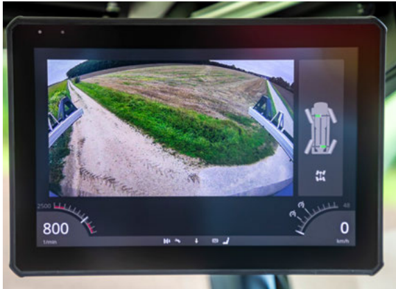
High-resolution, automatic display of the rearview camera in the A-column display
