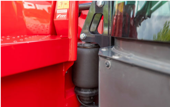
Pneumatic 4-point cabin suspension
