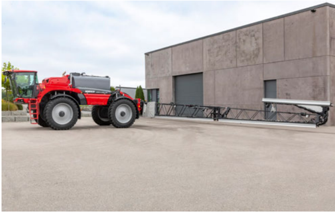
Optional: Hydraulic boom reduction 17/36 (m) to 30 m
