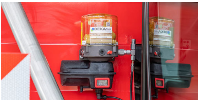
Tank of the central lubrication unit
