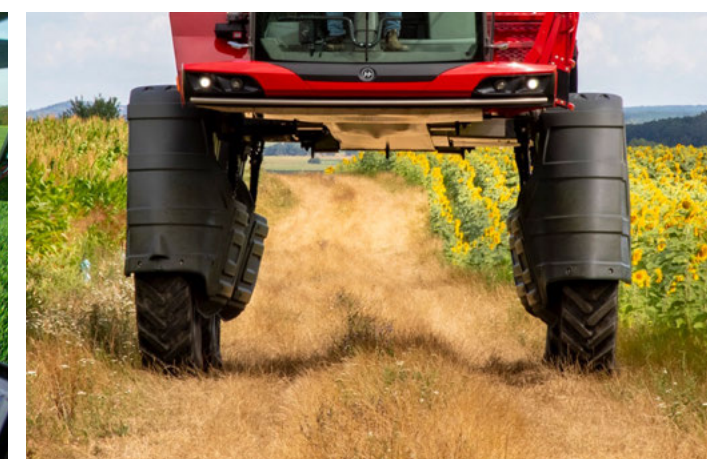
Highest clearance and a crop-protecting underbody
