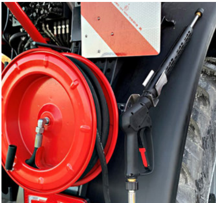
Hydraulically operated high-pressure cleaner
