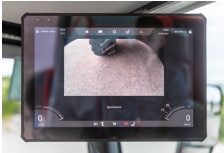
High-resolution, individual display of the track camera in the A-column display
