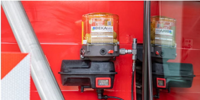
Tank of the central lubrication unit
