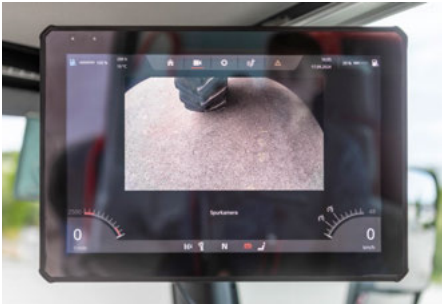
High-resolution, individual display of the track camera in the A-column display
