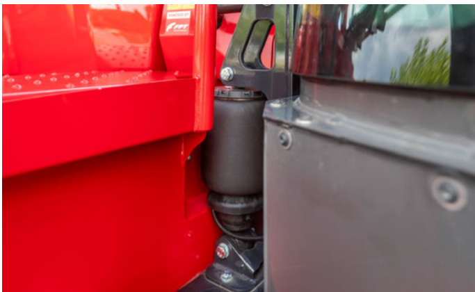
Pneumatic 4-point cabin suspension
