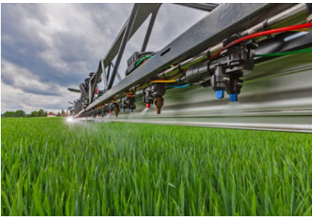
Pneumatic nozzle control 2-2
