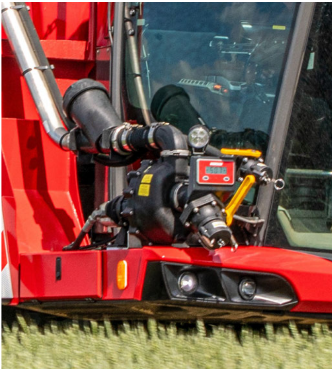
3" external fi ling connection including filter next to the cab
