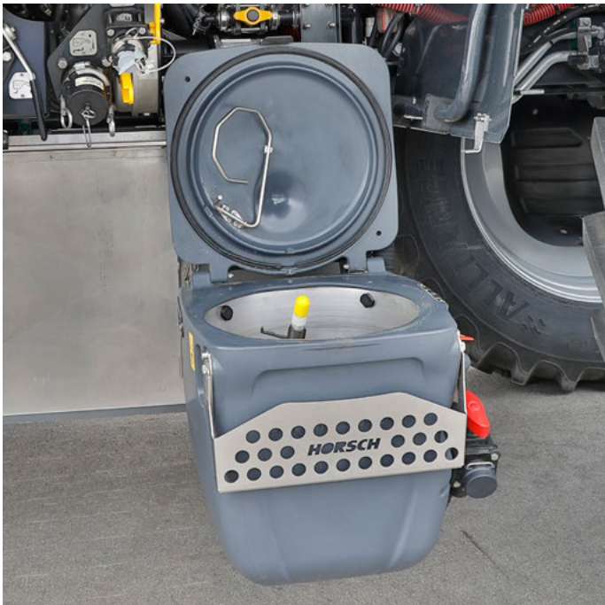
52 l stainless steel induction hopper incl. additional shock nozzle
