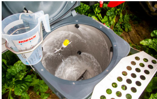
52 L stainless steel induction tank incl. additional impact nozzle
