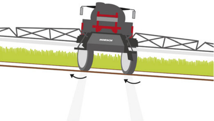
The active hillside counter-steering system HillControl compensates drift on side slopes and ensures a directionally stable following of the rear axle.
